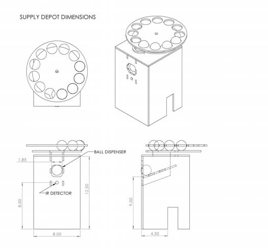
The re-supply depot will deliver a single ball each time its IR detector receives a series of 10 pulses with a 10ms ( $\pm 0.1$ ms) on time and a 30ms ( $\pm 0.1$ ms) off time. While delivering these pulses the ship must also illuminate a visible LED that is clearly visible to any observer.
